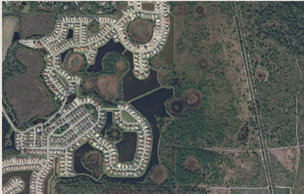
Stormwater management facilities for developments backing-up to managed environment areas can be strategically placed to create a barrier to developmental impacts such as lights, domestic cats, and children.
