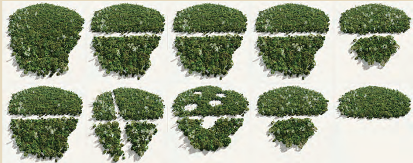
Habitat dissection (a road through it), fragmentation (multiple roads), dissection with perforations (roads and development sites), habitat dissection with shrinkage and finally attrition (overall loss or reduction of habitat).
