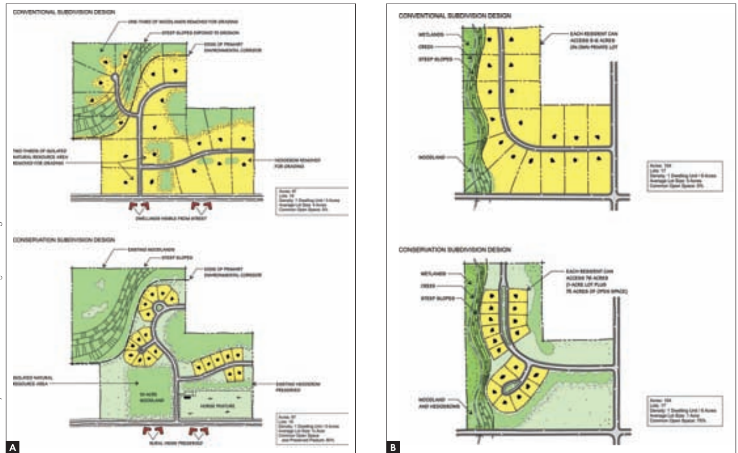
A) The same piece of land can be subdivided to better conserve the natural system, habitat and wildlife resources (bottom) or subdivided in what is commonly called conventional subdivision design (top).; B) Subdividing property judiciously to preserve the natural features and wildlife opportunities. The top illustration shows the traditional subdivision of land, while the bottom illustration has the same number of lots, but preserves the natural features and wildlife opportunities.
