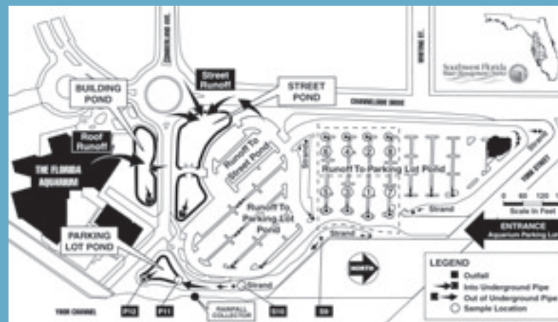
Figure 3.8. An integrated stormwater treatment train, including a wet detention pond, were used at the Florida Aquarium.
