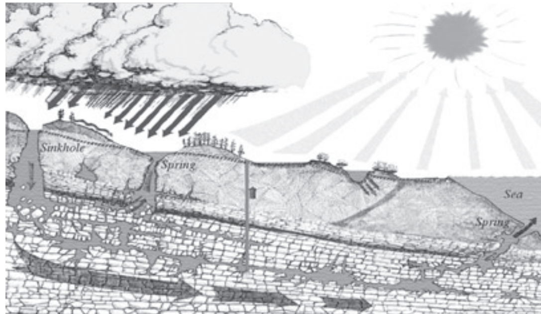
Figure 1.3. In a karst area, sinks and springs connect ground and surface waters.
